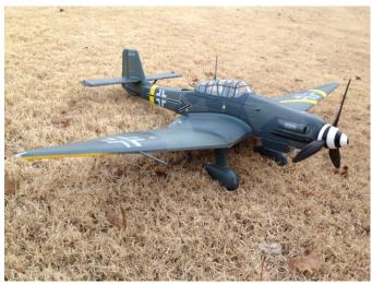
Total all up flying weight with a 4 cell 3300 mAh lipo comes in right at 80 ounces (Wing Area = 458 square inches). This comes in at the high end of the RC wing loading scale at 25 oz/square foot but I feel ("hope") that the plane will fly well with the included 3648-600KV Motor and 13x9 3 blade prop. I've done several run ups and the setup produces plenty of thrust! The Stuka and I look forward to seeing everyone at the next club meeting!
