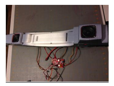
You could have the Stuka assembled and ready to fly in a matter of minutes without installing the sound system; however the addition of the sound system and LED's did complicate the build just a little bit. Some soldering and connector crimping was required and the sound board fits perfectly into the fuselage. After all was said and done there was little room left in the fuselage.
