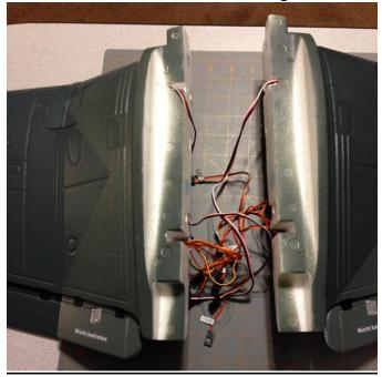
The engine startup, run and shut down sounds are tied to the throttle. I ended up using a 6 channel receiver and tied the dive siren sound and cannons to the flaps since the Stuka deployed full flaps before a dive bombing run. The machine guns are connected to a separate channel switch.
