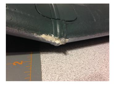
Next came the decision of where do I install the two speakers? After doing a little bit of research I decided to get out the foam cutter and remove foam from the chin scoop and the fuselage area just behind the leading edge of the wing. I then carefully applied a small amount of "Gorilla" glue to the speaker boxes and placed them into the cutouts. The rigidly mounted speaker boxes should take up for any structural integrity lost as a result of the foam removal.
